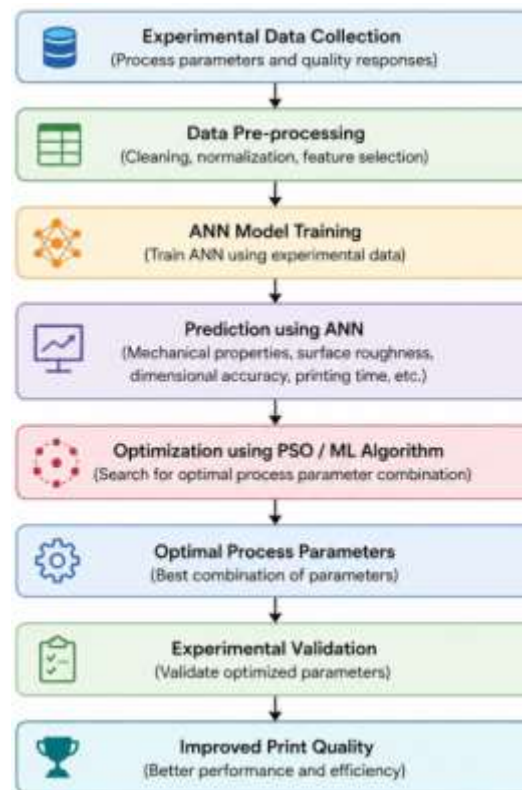
Figure 3: AI-Based Workflow for FDM Process Parameter Optimization
